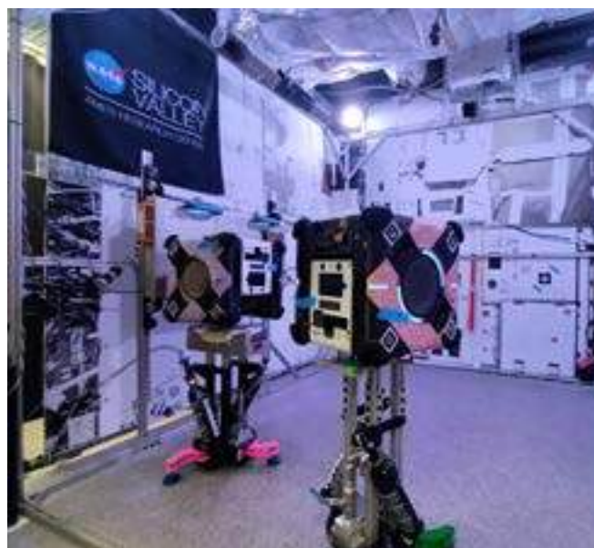
CSIRO's multi-resolution scanning payload attached to an Astrobee robot platform in a simulated ISS environment at NASA Ames Research Center. (CSIRO)
