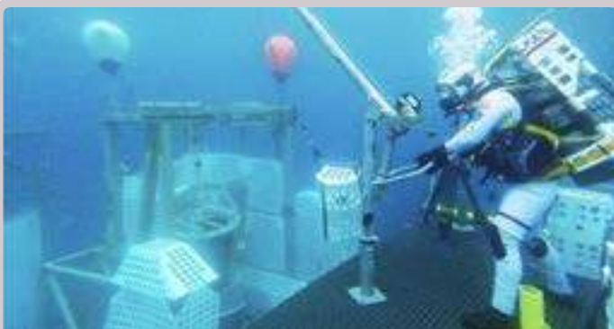
Testing methods for EVA crew-supported logistics handling on the Moon during SEATEST 6. (NASA)
