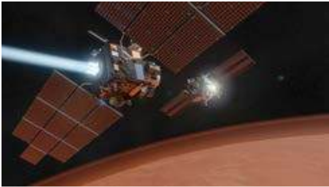
ESA's LightShip concept: A Mars Propulsive Tug capability building on Earth Return Orbiter technology, including communications and navigation services and science payloads. The LightShip can also deliver multiple scientific passenger spacecraft to Mars. (ESA)
