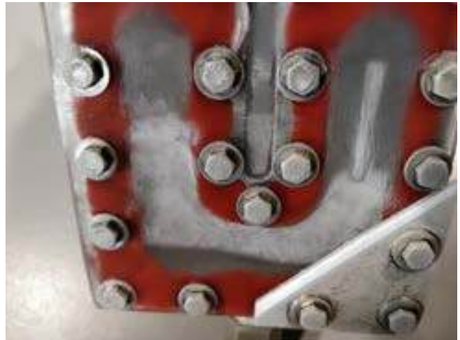
Water ice extracted from lunar regolith simulant trapped in a laboratory condenser during development of ASI's ORACLE. (ASTRA team – Politecnico di Milano)
