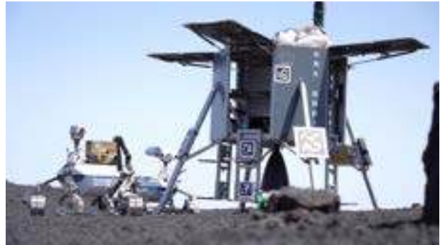
Two Lightweight Rover Unit (LRU) rovers pick up a modular payload from a lander in a cooperative mission scenario during the ARCHES analogue campaign at Mt. Etna, 2022 (DLR)
