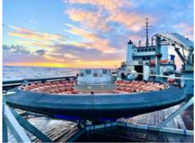
The 6-metre Low-Earth Orbit Flight Test of an Inflatable Decelerator flight test article on the recovery ship in November 2022, following a successful demonstration replicating Mars flight conditions. (NASA/Gregory Swanson)
