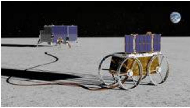
Lunar surface power systems will include converters, cables, and deployment devices. (Astrobotic)
