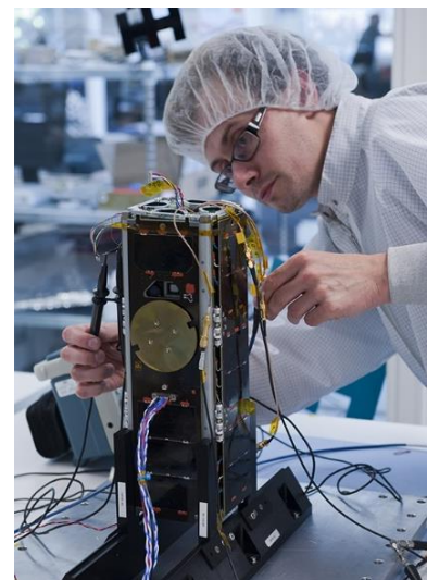
Figure 1: UKube-1 prepared for launch. This was UK's first official CubeSat, launched in 2014, and was built by Clyde Space Ltd in Glasgow. The 3U CubeSat, approximately 10cm x 10cm x 30cm and 3kg, carried 6 payloads.
