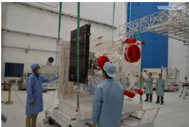
Figure 8: Micius Satellite being prepared for launch. The QUESS mission launched Micius in 2016 and successfully demonstrated a series of pioneering space quantum communication experiments. Micius has a mass of 650kg and is estimated to have cost USD100M in addition to the launch. Photo: Chinese Academy of Sciences
