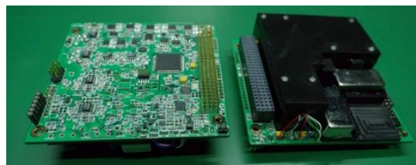
Figure 2: SPEQS-1 correlated photon pair source. The quantum payload is 10cm x 10cm x 3cm in size with a mass of 300g. It produces pairs of photons that possess the property of quantum entanglement that can be used for secure communication.
